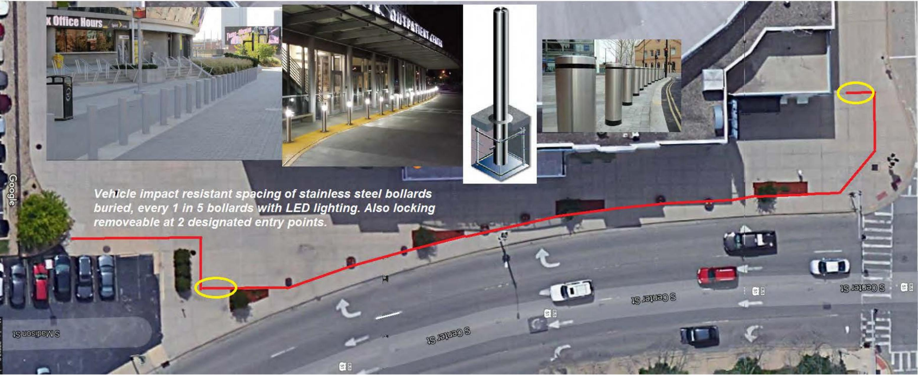
*Vehicle impact resistant spacing of stainless steel bollards buried, every 1 in 5 bollards with LED lighting. Also locking removeable at 2 designated entry points.*
