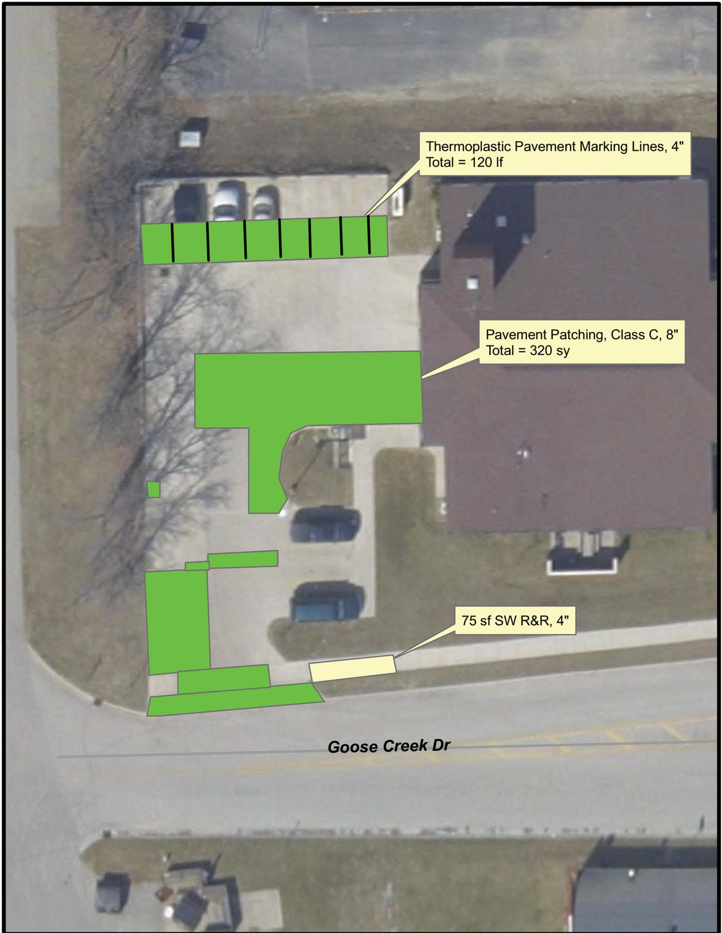
Thermoplastic Pavement Marking Lines, 4"
